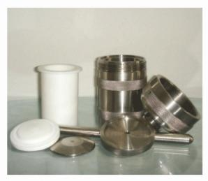
Hydrothermal synthesis reactor, also known as polymerization reactors, digestion tanks, high pressure digestion tank, pressure vessel, reactor, pressure container bombs, digestion tanks, hydrothermal synthesis reactor, experiment reflects the kettle.
